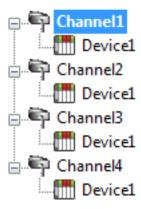
Each device has now been defined under its own channel. In this new configuration, a single path of execution is dedicated to the task of gathering data from each device. If the application has 256 or fewer devices, it can be optimized exactly how it is shown here.
