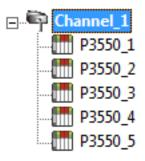
Each device appears under a single AutomationDirect Productivity Series Ethernet Driver channel. In this configuration, the driver must move from one device to the next as quickly as possible in order to gather information at an effective rate. As more devices are added or more information is requested from a single device, the overall update rate begins to suffer.
