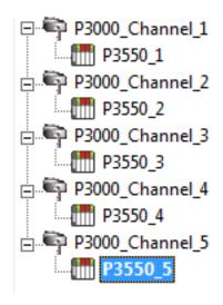
Each device has now been defined under its own channel. In this new configuration, a single path of execution is dedicated to the task of gathering data from each device. If the application has 256 or fewer devices, it can be optimized exactly how it is shown here.
