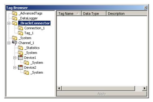
To select a Server Tag, double-click on it. Alternatively, highlight it and then press **Apply**. This will return the Server Tag to the connector.
