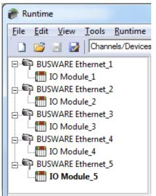
Each device has now been defined under its own channel. In this new configuration, a single path of execution is dedicated to the task of gathering data from each device. If the application has 16 or fewer devices, it can be optimized exactly how it is shown here
