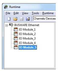
Each device appears under a single Busware Ethernet channel. In this configuration, the driver must move from one device to the next as quickly as possible in order to gather information at an effective rate. As more devices are added or more information is requested from a single device, the overall update rate begins to suffer.
