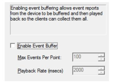
• **Enable Event Buffer:** When checked, this option allows event reports from the remote DNP device to be buffered and played back for OPC client collection. The default setting is unchecked.
