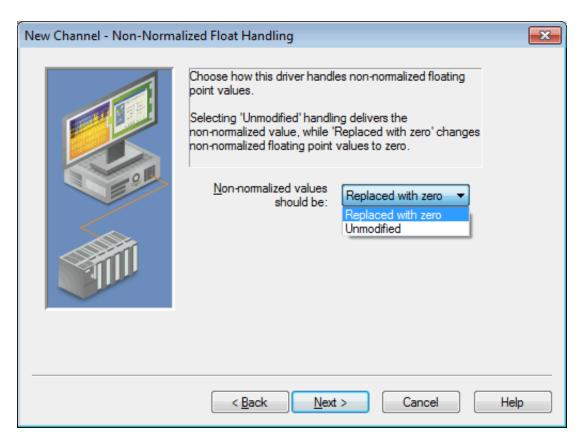
**Replaced with zero** recognizes invalid outliers and eliminates them by replacing the value with integer zero (default).
