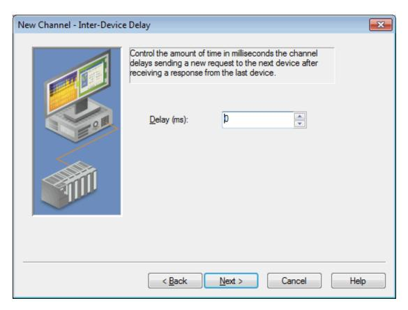
**Delay** Accept 0 milliseconds (default) or adjust using the up/down arrows. The range is 0-60000 ms.
