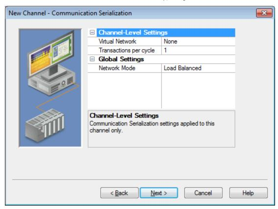
**Virtual Network** - Select the network name or the default, None **Transactions per cycle** - Enter the target number or accept 1 (default). **Network Mode** -Select Priority or Load Balanced (default).
