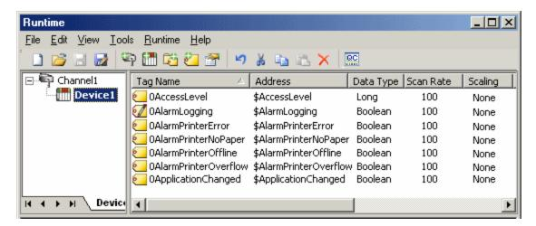
**Note:** Generated tag names are essentially the same as the tag names in InTouch. Minor name modifications may be required and are indicated in the Event Log when they occur. The addresses in the OPC server are the same as the tag names in InTouch.
