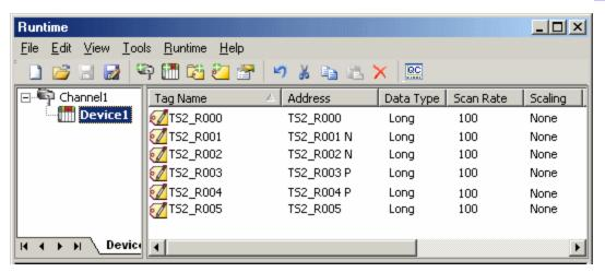
In this example, tags TS2\_R001 and TS2\_R002 are placed in Notified Mode regardless of the device-level settings. Tags TS2\_R003 and TS2\_R004 are placed in Polled Mode regardless of the device-level settings. All other tags shown above use the default mode specified in Device Properties.
