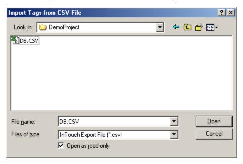
In this example, the file in an InTouch project folder called "DB.CSV" has been selected. Once  $\mathbf{OK}$  is clicked, the full path and file name is automatically placed in the InTouch CSV file box.
