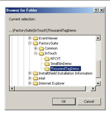
In this example, the root folder of an InTouch project called "ThousandTagDemo" has been selected. Once **OK** is clicked, the full path to this folder is automatically placed in the InTouch project folder box.
