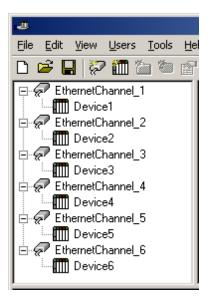
Each device has now been defined under its own channel. In this new configuration, a single path of execution is dedicated to the task of gathering data from each device. If the application has 256 or fewer devices, it can be optimized exactly how it is shown here.
