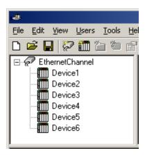
Each device appears under a single Opto 22 Ethernet Device channel. In this configuration, the driver must move from one device to the next as quickly as possible in order to gather information at an effective rate. As more devices are added or more information is requested from a single device, the overall update rate begins to suffer.
