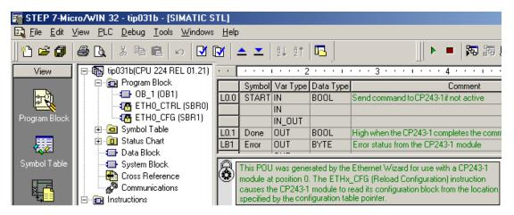
5. Now that the results of the Ethernet wizard have been confirmed, a connection can be made using the OPC server.
