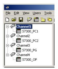
Each device has now been defined under its own channel. In this new configuration, a single path of execution is dedicated to the task of gathering data from each device.
