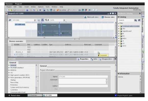
11. Once finished, view the project tree. Locate **Program Blocks** and **PLC Tags** and then configure the addresses that will be used in the PLC project.
