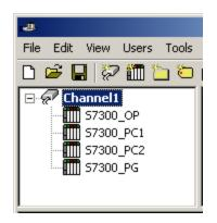
Each device appears under a single Siemens TCP/IP Ethernet channel. In this configuration, the driver must move from one device to the next as quickly as possible to gather information at an effective rate. As more devices are added or more information is requested from a single device, the overall update rate begins to suffer.
