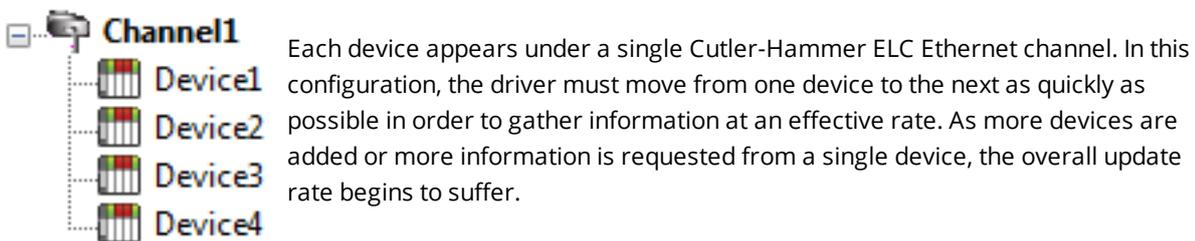
If the Cutler-Hammer ELC Ethernet Driver driver could only define one single channel, then the example shown above would be the only option available; however, the Cutler-Hammer ELC Ethernet Driver driver can define up to 256 channels. Using multiple channels distributes the data collection workload by simultaneously issuing multiple requests to the network. An example of how the same application may appear when configured using multiple channels to improve performance is shown below.
