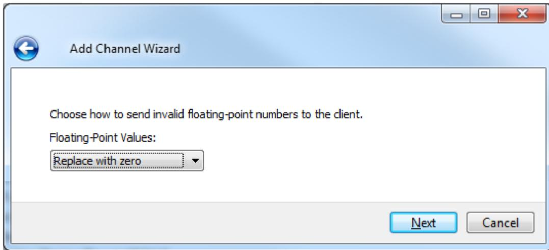
**Replaced with zero** recognizes invalid outliers and eliminates them by replacing the value with integer zero (default).
