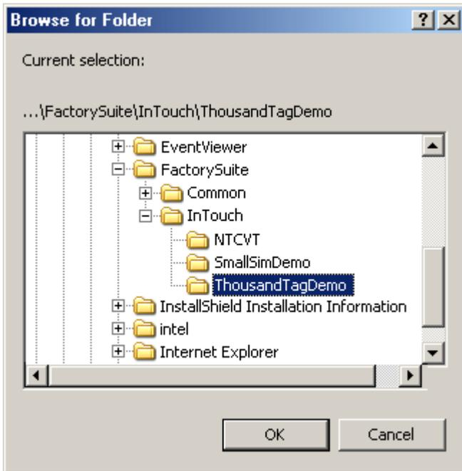
In this example, the root folder of an InTouch project called "ThousandTagDemo" has been selected. Once **OK** is clicked, the full path to this folder is automatically placed in the InTouch project folder box.
