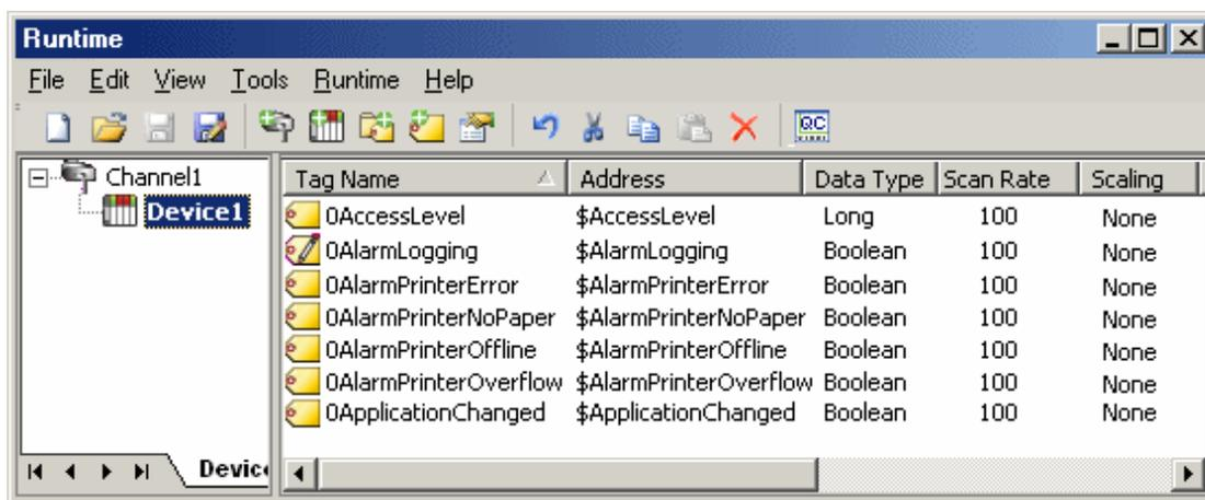
**Note:** Generated tag names are essentially the same as the tag names in InTouch. Minor name modifications may be required and are indicated in the Event Log when they occur. The addresses in the OPC server are the same as the tag names in InTouch.
