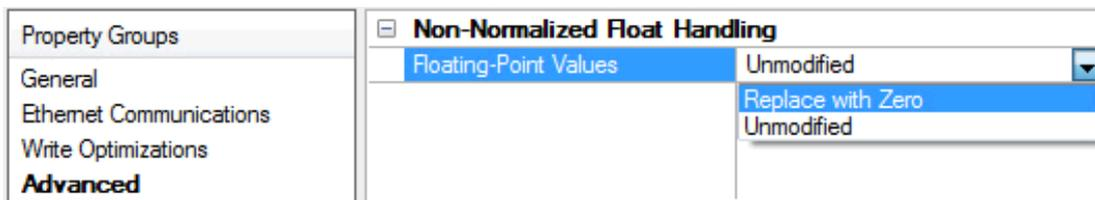
**Non-Normalized Float Handling:** Non-normalized float handling allows users to specify how a driver handles non-normalized IEEE-754 floating point data. A non-normalized value is defined as Infinity, Not-a-Number (NaN), or as a Denormalized Number. The default is Replace with Zero. Drivers that have native float handling may default to Unmodified. Descriptions of the options are as follows:
