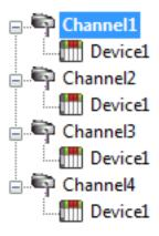
Each device has now been defined under its own channel. In this new configuration, a single path of execution is dedicated to the task of gathering data from each device. If the application has 16 or fewer devices, it can be optimized exactly how it is shown here.
