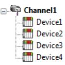
Channel1Each device appears under a single IOtech PointScan 100 driver channel. In this<br/>configuration, the driver must move from one device to the next as quickly as<br/>possible in order to gather information at an effective rate. As more devices are<br/>added or more information is requested from a single device, the overall updateDevice3Device3
