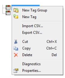
Tag groups can be added at any level from the device-level down, and multiple tag groups can be nested together to fit the application's needs. As seen in the OPC Quick Client dialog above, the fully qualified OPC item path is "Channel1.Device1.Machine1.Cell1.Tag1". For this OPC item, "Machine1" and "Cell1" segments are nested tag groups.
