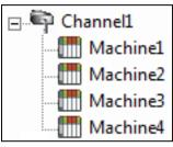
Each device appears under a single channel. In this configuration, the driver must move from one device to the next as quickly as possible to gather information at an effective rate. As more devices are added or more information is requested from a single device, the overall update rate begins to suffer.
