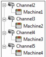
Each device has now been defined under its own channel. In this new configuration, a single path of execution is dedicated to the task of gathering data from each device. If the application has fewer devices, it can be optimized exactly how it is shown here.
