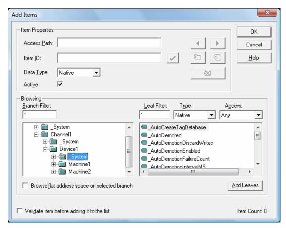
The \_System branch found under the DeviceName branch is always available. If referencing a system tag from a DDE application given the above example and the DDE defaults, the link would appear as "<DDE service name>|\_ddedata!Channel1.Device1.\_System.\_Error".
