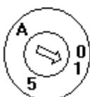
For models of the AJ71C24 which support multidrop operation, the Station Number must be set between 0 and 31.
