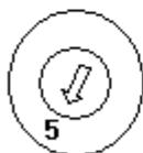
The AJ71C24R4 MUST be set for Protocol 1. This means the Mode switch must be set to position 5.
