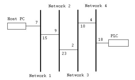
The Host PC's address from the PLC's perspective is 4.2.9.7.1. The PLC's address from the Host PC's perspective is 15.23.10.18.0. This is the Device ID path. If the same registers were transferred from the PLC to the same locations in the Host PC, the following control block and data area would be used in the MSTR instruction:
