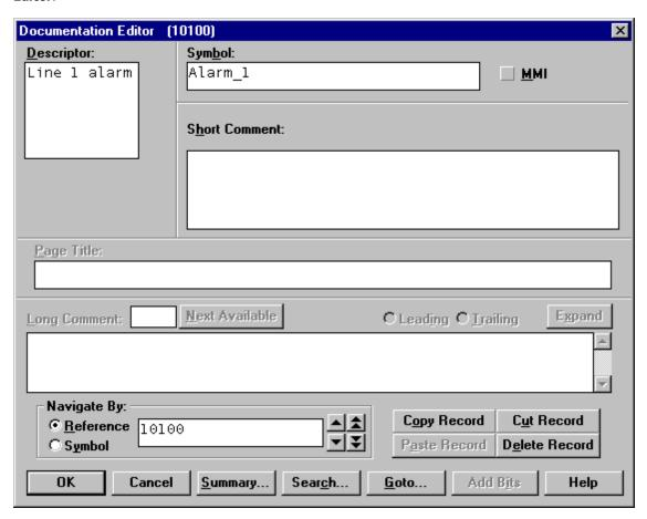
**Note:** ProWORX does not place many restrictions on variable names. The OPC Server, however, requires that tag names consist of only alphanumeric characters and underscores, and that the first character not be an underscore. The driver will modify invalid imported tag names as needed will inform when any name changes in the server's Event Log.
