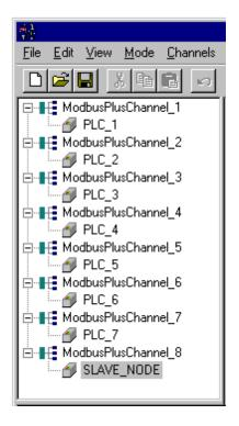
Each device has now been defined under its own channel. In this new configuration, the OPC Server can dedicate a single path of execution to the task of gathering data from a single device because each has its own dedicated channel. If the application has 8 or less devices it can be optimized as displayed.
