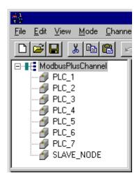
In this project, there is only one Modbus Plus channel defined. All devices that need to be accessed are defined under that one channel. Thus, the Modbus Plus Driver must move from one device to the next as quickly as possible to gather information at an effective rate. As more devices are added or more information is requested from a single device, the update rate begins to suffer.
