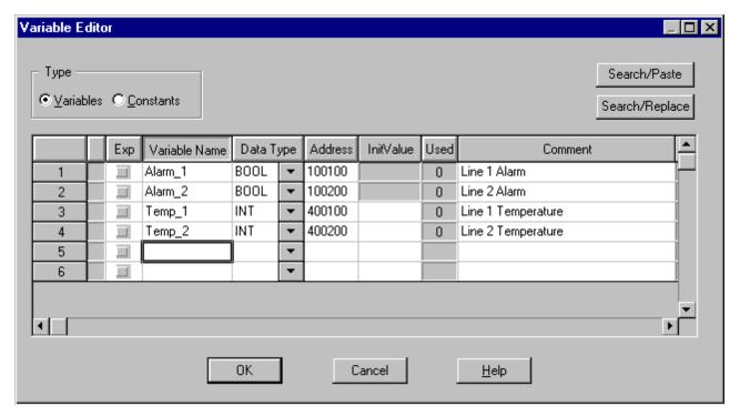
**Note:** Although Concept can define variable names that begin with an underscore, such names are not allowed by the OPC server. The driver will modify invalid imported tag names as needed and note all name changes in the server's Event Log.
