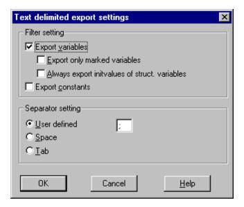
**Note:** Although any filter settings can be chosen, this driver will only be able to read the exported data if the default semicolon separator is used.
