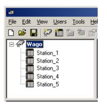
Each device appears under a single Wago Ethernet channel. In this configuration, the driver must move from one device to the next as quickly as possible in order to gather information at an effective rate. As more devices are added or more information is requested from a single device, the overall update rate begins to suffer.
