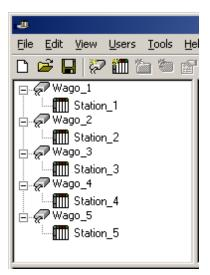
Each device has now been defined under its own channel. In this new configuration, a single path of execution is dedicated to the task of gathering data from each device. If the application has 16 or fewer devices, it can be optimized exactly how it is shown here.
