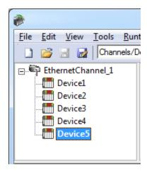
Each device appears under a single Yokogawa DXP Ethernet Driver channel. In this configuration, the driver must move from one device to the next as quickly as possible in order to gather information at an effective rate. As more devices are added or more information is requested from a single device, the overall update rate begins to suffer.
