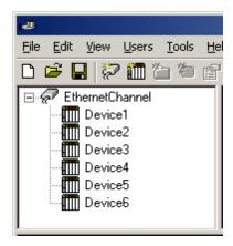
Each device appears under a single Yokogawa MX Ethernet Device channel. In this configuration, the driver must move from one device to the next as quickly as possible in order to gather information at an effective rate. As more devices are added or more information is requested from a single device, the overall update rate begins to suffer.
