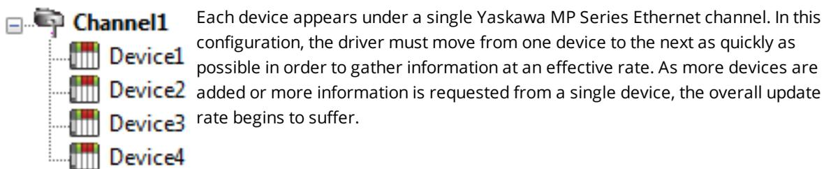
If the Yaskawa MP Series Ethernet Driver could only define one single channel, then the example shown above would be the only option available; however, the Yaskawa MP Series Ethernet Driver can define up to 16 channels. Using multiple channels distributes the data collection workload by simultaneously issuing multiple requests to the network. An example of how the same application may appear when configured using multiple channels to improve performance is shown below.
