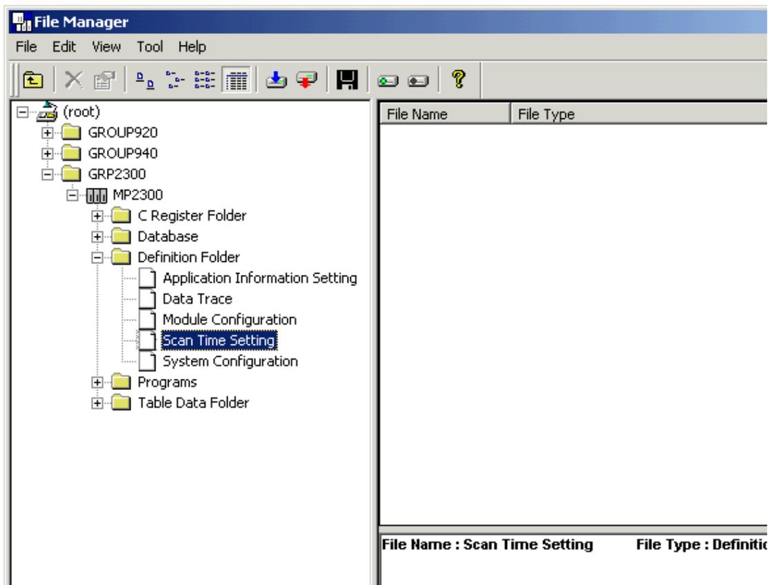
4. In **Scan Time**, note the **High Speed Scan Setting** and **Low Speed Scan Setting** fields. Yaskawa recommends 1ms for the High Scan setting and 20ms for the Low Scan setting.
