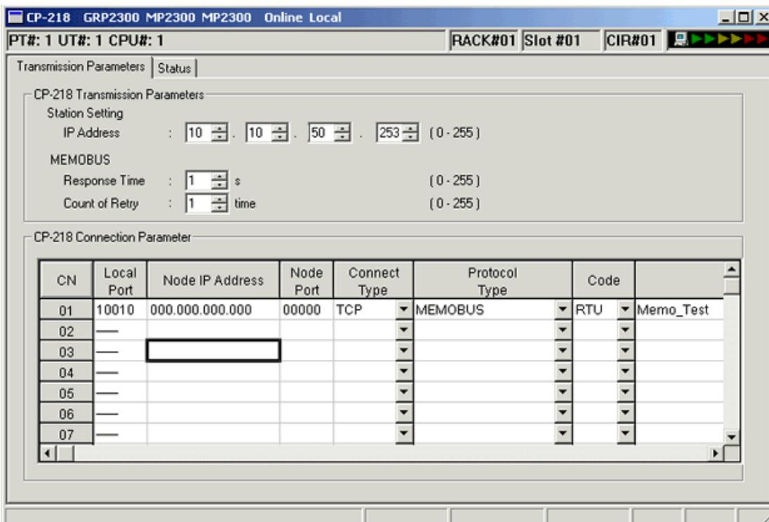
10. If there is the possibility of a device connection from another LAN, set the **Network Subnet Mask** and **Gateway IOP Address**. To do so, select **Edit | Local Port: TCP/IP Setting** from the **File Manager** main menu. In the **Station Setting** dialog, set the Subnet Mask and Gateway IP values. Then, click **OK** to set and close.
